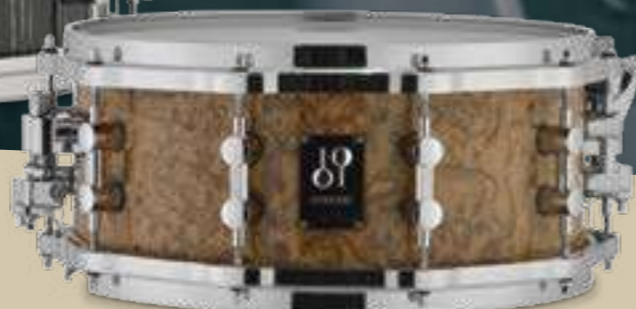
14" x 6" Maple Snare in Chocolate Burl (PL 12 1406 SDWD) 20 tension rods, TuneSafe, die-cast hoops, 9 ply Vintage Maple shell, 4 mm thickness plus 2 mm reinforcement rings, 45° bearing edge
