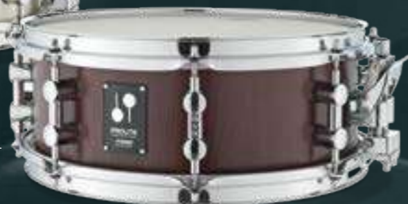
13" x 5" Maple Snare in Nussbaum (PL 12 1305 SDW) 16 tension rods, TuneSafe, 2.3 mm Power Hoops, 9 ply Vintage Maple shell, 4 mm thickness plus 2 mm reinforcement rings, 45° bearing edge
