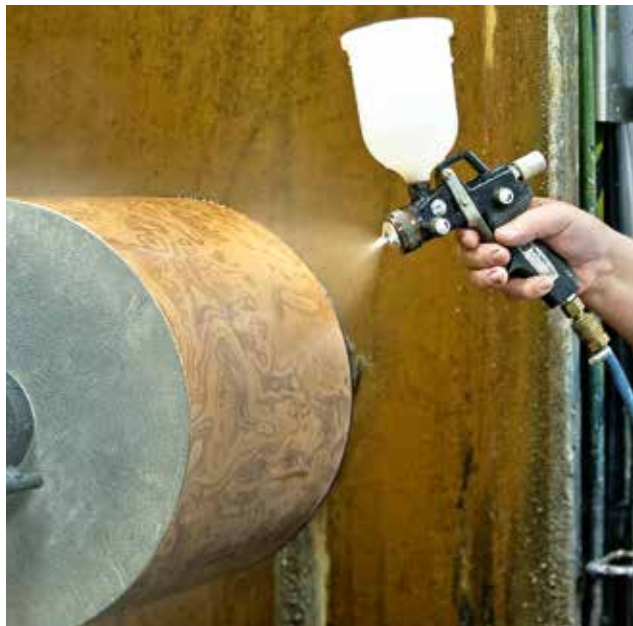
Precision lacquering is applied to protect the exclusive natural wood finishes or the multiple layers of high quality colour finishes.
