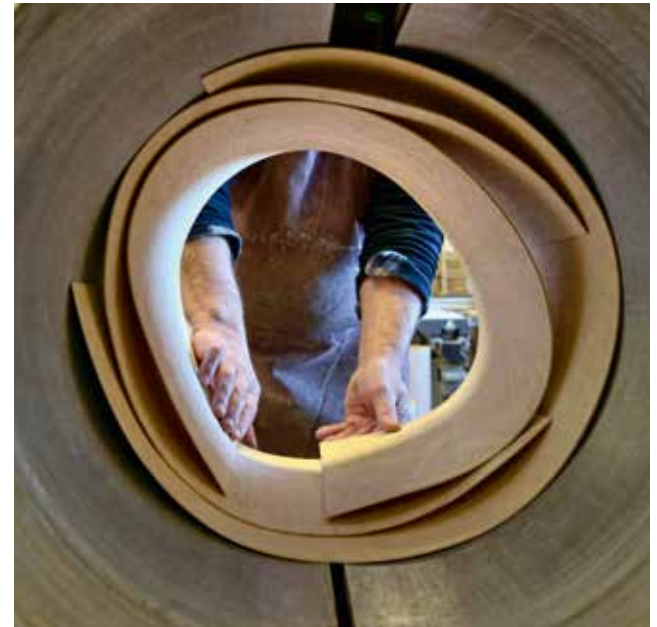
CLTF stands for Cross Laminated Tension Free – a process that gives each shell superior stability and acoustic quality and requires no internal pressure on the shell.
