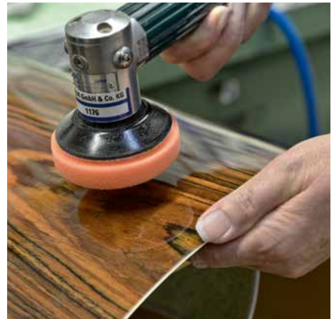
Hand polishing ensures a perfect finish of each drum shell and the outstanding looks that are a hallmark of Sonor instruments.
